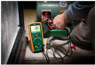
Insulation test on pump motor
