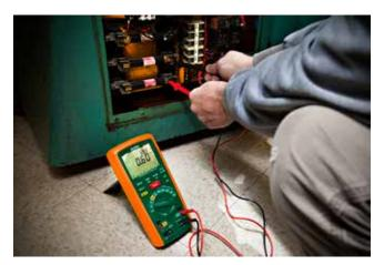
Checking voltage on a lathe
