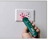
Check voltage in breakers and outlets
