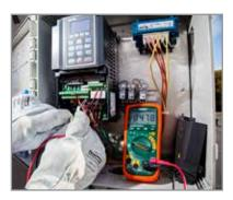
Low Past Filter (LPF) ensures accurate AC Voltage measurements on a variable frequency drive.
