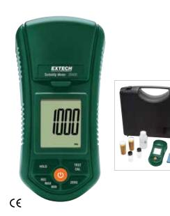
Complete with all the accessories to conveniently test the turbidity of municipal water, food and beverage water, and other aqueous solutions where fluid clarity is important
