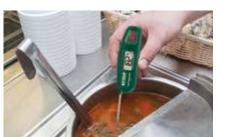
2.4" (61mm) folding stainless steel probe (NSF certified) for measuring in liquids, pastes, and semi-solid food. Ideal for use in food industry, agriculture, and laboratories.
