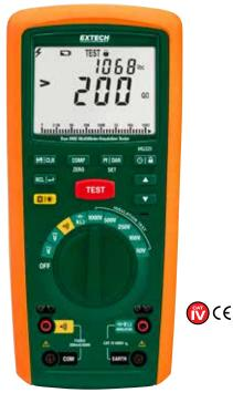
Includes test leads, alligator clip, remote probe with built-in test button, 6 x AA batteries, and soft case. High Insulation Resistance range ( $200G\Omega$ ) and fully loaded DMM functions. Combines a  $200G\Omega/1000V$  high range Insulation Tester with a full-featured True RMS MultiMeter in a single, compact instrument. CAT IV safety rating ensures the highest level of protection.
