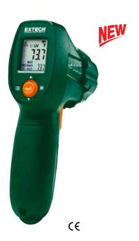
Adjustable emissivity for better accuracy on different surfaces
