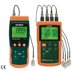
Includes remote vibration sensor(s) with magnetic adapter, batteries, SD card, and hard case; SDL800 has 3yr warranty and optional AC Adaptor. VB500 has 2yr warranty and also includes 4 vibration sensors and 100-240V Universal AC Adaptor.
