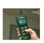
Measure CO<sub>2</sub> level in office buildings to ensure proper ventilation. Includes software and cable, 4 AA batteries, and case; 2 years warranty
